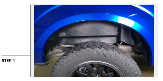
Tighten all the Phillips screws, repeat procedure for other side.
