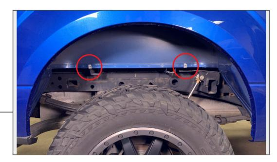
Install (2) U-Clips into the pre-drilled locations inside the wheel well.
