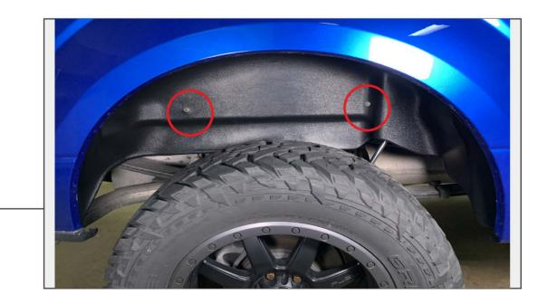
Place the wheel well liner into the vehicle. Install (2) Phillips screws into the fender liner, but do not tighten.
