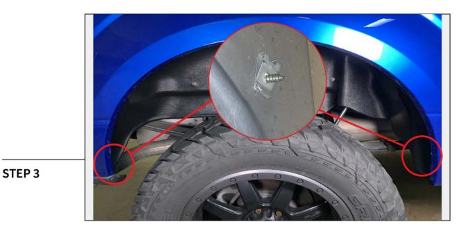
Using (2) U-Clips as nuts, install (2) Phillips screw into the fender liner. The U-Clip goes behind the sheet metal of the wheel well. Hold the U-Clips in place with pliers while tightening.
