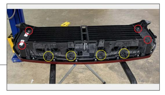
Remove the (4) push clips at the top of the grille, then the (4) 8mm nuts at the bottom. Remove inner assembly from the grille and transfer it to the new grille.
