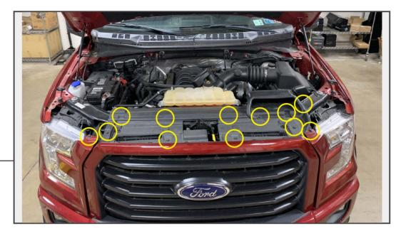
Using a panel removal tool, remove (12) push clips to remove the plastic radiator cover from the grille.
