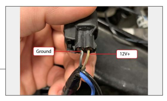
Route the grille light wiring to the passenger side headlight. Tap into the parking light connector using (2) provided Scotch-Locks following the diagram below. Confirm lighting works before reassembly.
