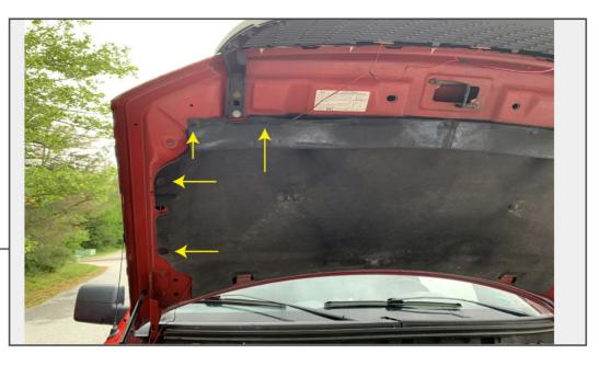
Remove (4) push clips using a panel removal tool to gain access behind the hood insulation pad. Route the grille wiring behind the hood insulation pad, then towards the passenger side headlight.
