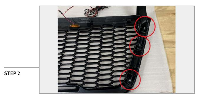
Install the grille mounting arms to the new grille using the provided (3) Phillips screws per side.
