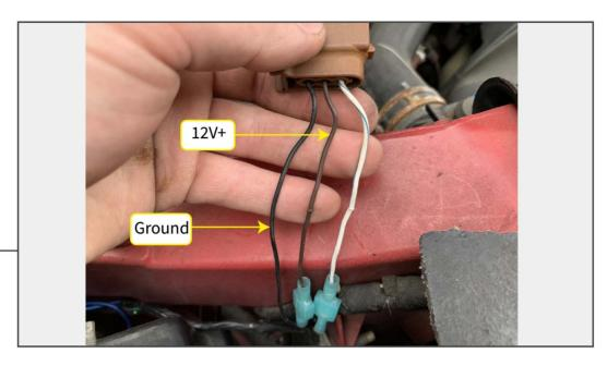
Unplug the turn signal harness. Using provided Scotch-Locks, tap into the parking light harness to power the lights. Be sure grille lights work before fully reassembly.
