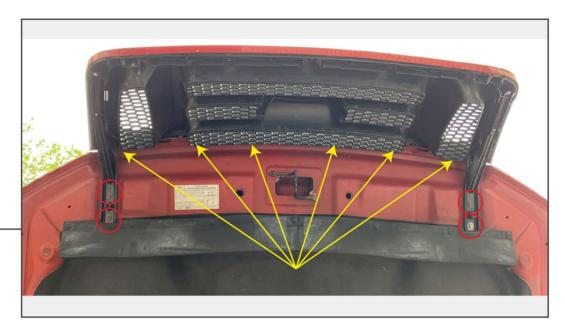
Begin by removing (4) 10mm Bolts, as well as (6) 10mm nuts. Lift and remove the grille from the vehicle.
