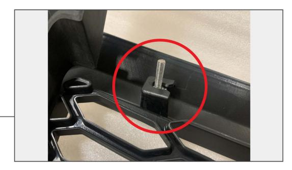
Using (6) provided studs, insert the studs behind the tabs along the top of the grille. Re-align grille to the vehicle.
