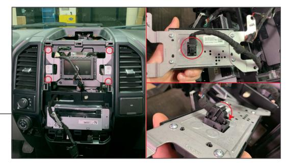
With the dash panel removed, use a 7mm socket to unscrew the (4) screws securing the factory display to the vehicle. Disconnect the (1) electrical plug from the unit.
