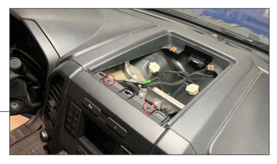
Using a 7mm socket, remove the (2) screws securing the factory trim panel to the vehicle.
