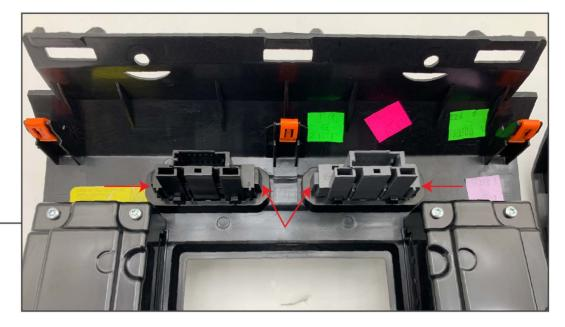
Transfer the Hazard and Traction control buttons from the factory trim panel to the Navos panel. Depress the tabs on the buttons and push them out of the panel. Transfer the buttons to the Navos panel.
