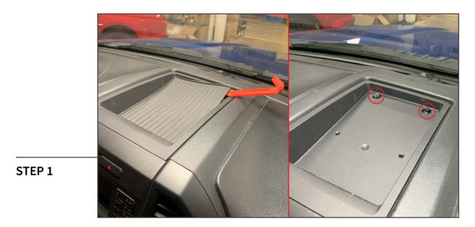
Using a soft pry tool, remove the rubber liner from the dash storage tray. Using a 7mm socket, remove the (2) screws.
