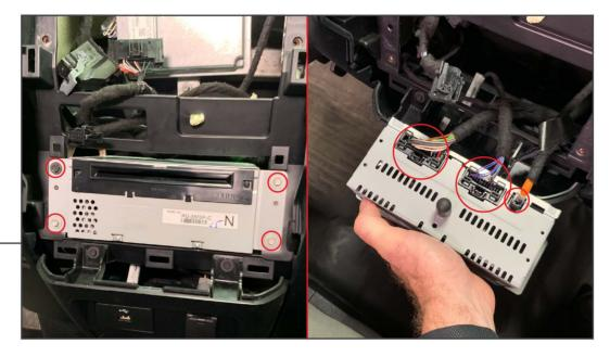
Using a 7mm socket, remove the (4) screws securing the factory CD/radio to the vehicle. Disconnect the (3) electrical plugs on the back of the unit.
