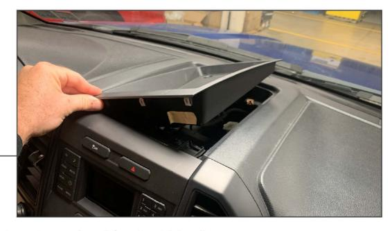
Pull up on the storage tray to release it from its retaining clips.
