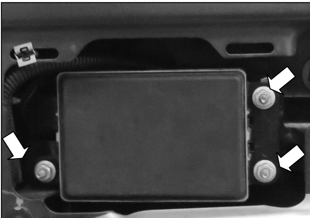
(Fig 3) Remove and unplug adaptive cruise control from driver/left side of frame, if equipped
