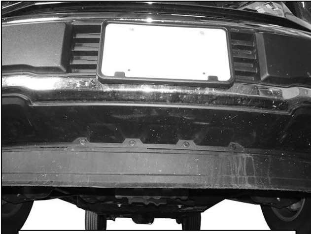
(Fig 1) Remove license plate from Bumper
