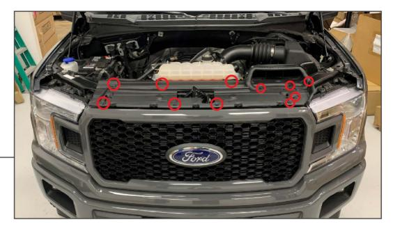
Remove (11) push clips from the upper splash shield. Remove upper splash shield from vehicle.
