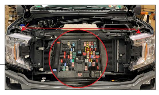
Route the provided DRL wiring harness neatly from the fuse box, across the engine bay to both headlight assemblies. Replace the indicated fuse with the DRL harness.
