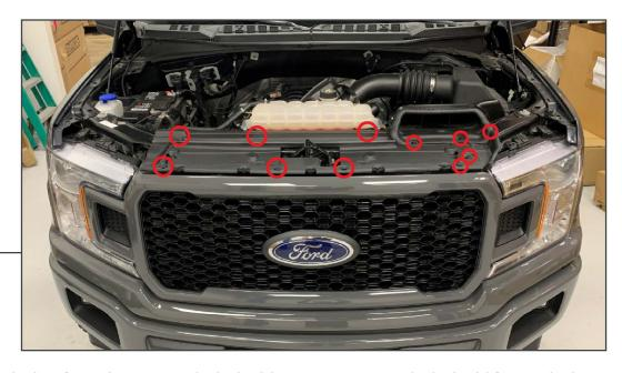
Remove (11) push clips from the upper splash shield. Remove upper splash shield from vehicle.
