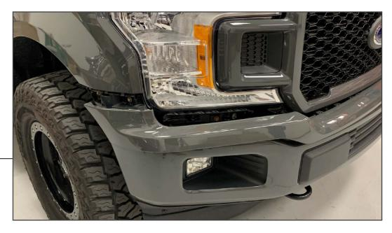
Firmly pull the trim panel away from the vehicle to dislodge the clips. Repeat this procedure to the opposite side. Remove the trim panel from the vehicle.
