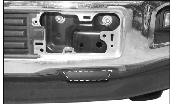
(Fig 12) Models without tow hooks, Cut slot through plastic splash guard to clear Support Bracket
