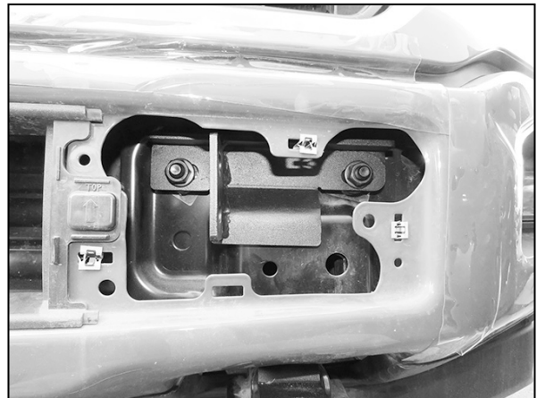
(Fig 8) Driver/left Frame Bracket installed
