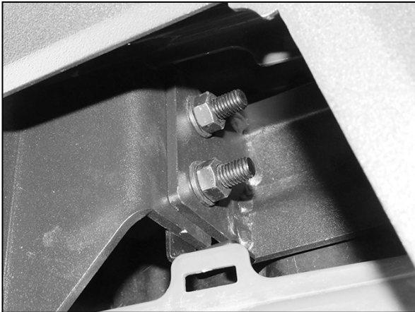
(Fig 19) Driver/left side of Bumper attached to "L" Double Bolt Plate and Bracket
