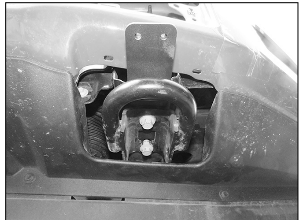
(Fig 14) Support Bracket installed between tow hook and bottom of frame
