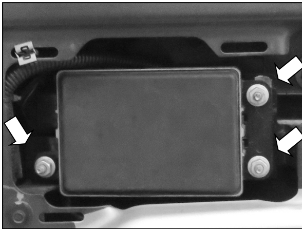
(Fig 3) Unplug and remove ACC sensor from driver/left side of bumper, if equipped
