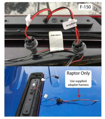
**Step 3\\**Take the new Axial light, and install the two light harnesses into the factory light bulb sockets. Install the brake light wire into the middle socket. The cab light can be installed into either end socket. Test for proper function.
