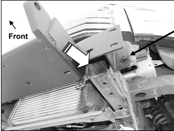
(Fig 11) Models without tow hooks, insert the included 12mm Double Nut Plate into open end of frame (arrow)
