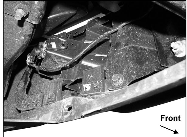
(Fig 4) Unplug and move factory wiring harness for fog lights (if equipped)
