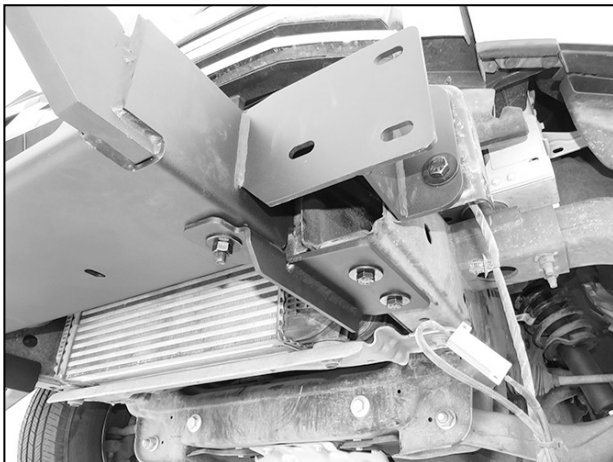
(Fig 13) Driver/left Support Bracket installed
