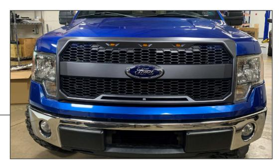
Slowly close the hood. If the grille is not centered between the headlights, slight adjustment is necessary. Refer to step 7, by loosening the nuts and adjusting the grille side to side.
