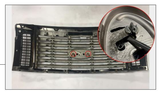
Remove (2) 10mm nuts securing the emblem to the grille. Using a flathead screwdriver, pry back on the emblem backing panel and release the emblem studs from the grille. Remove emblem through the front of the grille.
