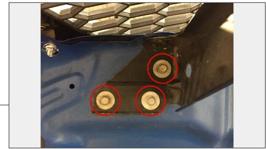
Using the (6) factory bolts, secure the grille brackets to the hood.
