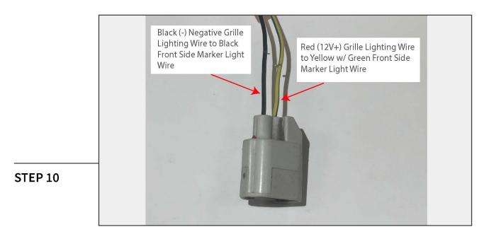
Using the (2) scotchlok connectors, splice the grille marker light wiring into the factory wiring as follows:
