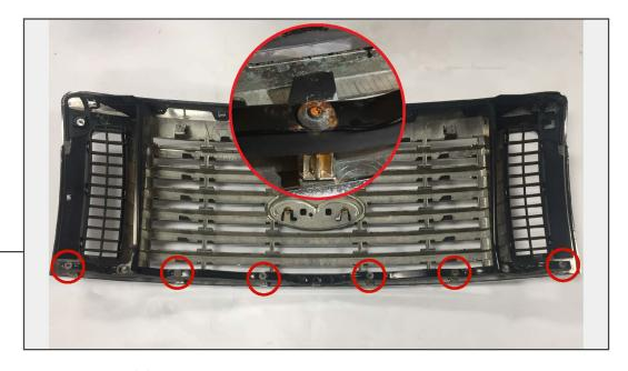
Using a T-25 torx bit, remove the (6) screws holding the grille brace to the factory grille.
