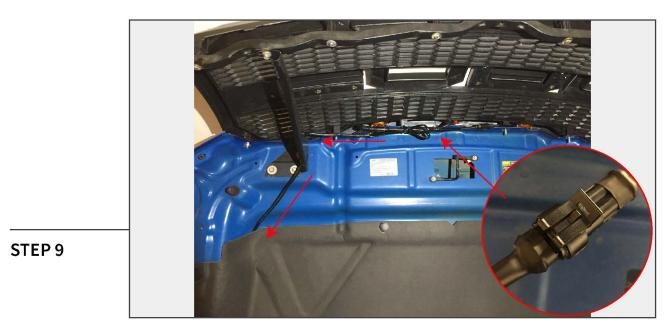
Connect the supplied wiring harness into the (3) LED grille marker lights. Zip tie the wiring safely along the hood insulation away from moving and/or hot engine components.
