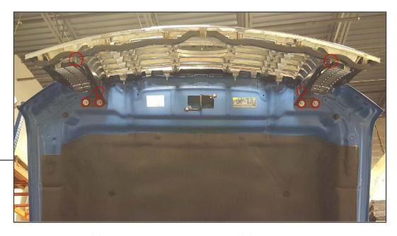
Using a 10mm socket, remove the (2) bolts across the top, and the (6) bolts holding the grille brackets to the hood. Remove bracket.
