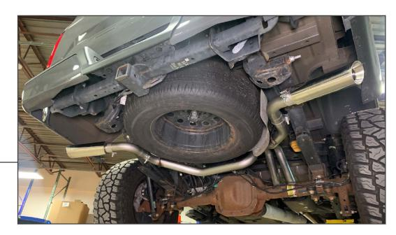
With the exhaust loosely installed, tighten all of the exhaust clamps. Work from the 2 bolt flange towards the exhaust tips. Rotate the muffler/pipes as need for best fit. Torque the 3/8-16 and exhaust tip fasteners to 25ft.-lbs. Tighten the exhaust clamps to 45ft.-lbs.
