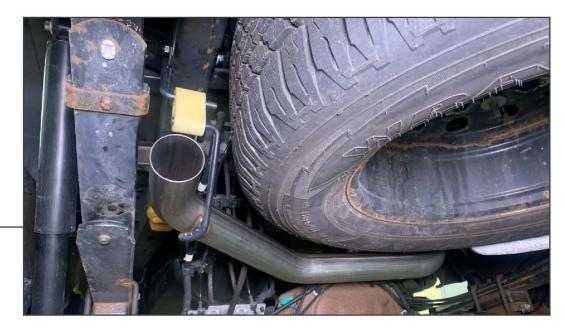
Hang the left side exhaust pipe using the provided isolator and hanger installed in step 3. Press the included star washers onto the hangers to keep the pipe centered and secured.
