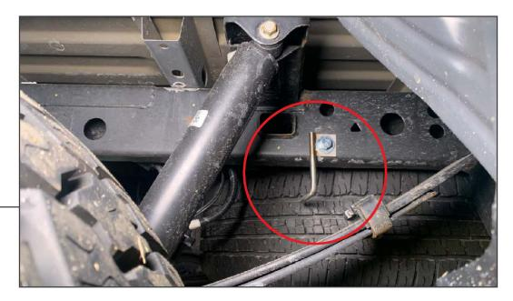
Install the supplied exhaust hanger using the provided M10x1.50 x 100mm bolt, flat washer, lock washer, square washer and hex nut. Torque to 25ft.-lbs.
