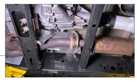
Lift and supporting the vehicle to gain access to the factory exhaust system. Locate the factory (2) bolt exhaust flange located to the right of the transmission/transfer case. Use a 13mm socket to remove the factory bolts.
