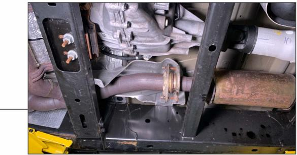
Begin by raising and supporting the vehicle to gain access to the factory exhaust system. Locate the factory (2) bolt exhaust flange located to the right of the transmission/transfer case. Use a 13mm socket to remove the factory bolts.
