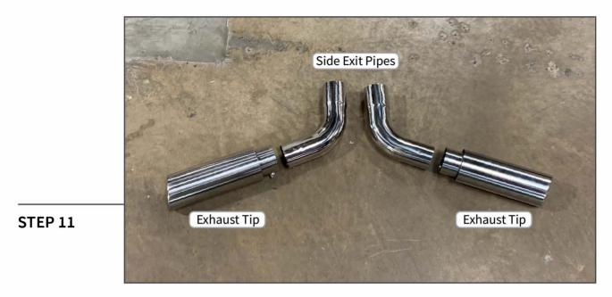
If the vehicle is equipped with a trailer hitch the side exit pipes must be used as shown above.
