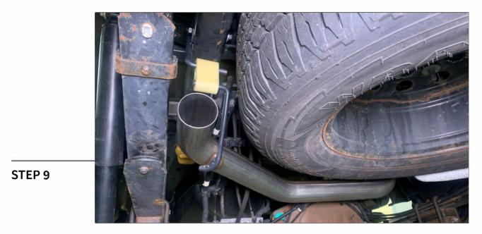
Hang the left side exhaust pipe using the provided isolator and hanger installed in step 3. Press the included exhaust hanger washers onto the hangers to keep the pipe centered and secured.
