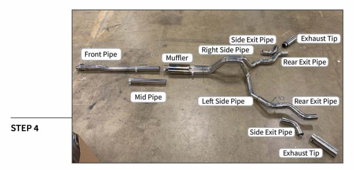
Identify the different exhaust components. Depending on your vehicles configuration, you may need to trim the front/mid pipe. See step 5.
