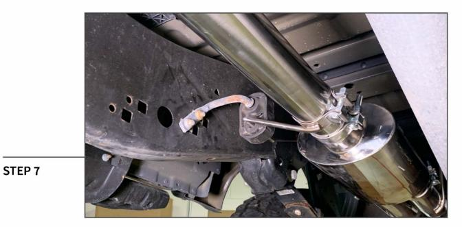
If required. slide the mid pipe onto the front pipe with an exhaust clamp. Then, install the clamp hanger so that it aligns with the factory frame mounted exhaust hanger right before the muffler. Reuse the factory rubber isolator and bolts.
