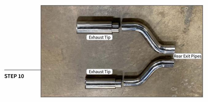
If the vehicle does not come equipped with a trailer hitch, the rear exit pipes may be installed. If the vehicle has a trailer hitch skip to step 11
