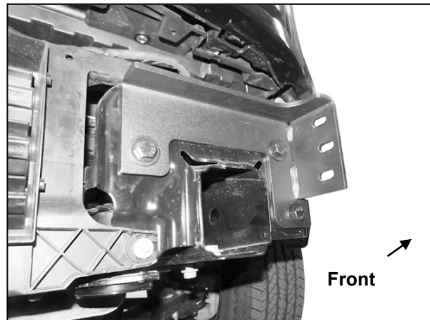
(Fig 8) Driver/left side Bracket installed
