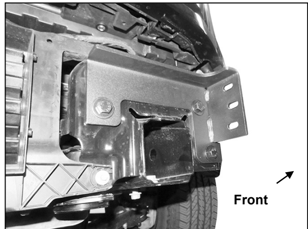
(Fig 8) Driver/left side Bracket installed
