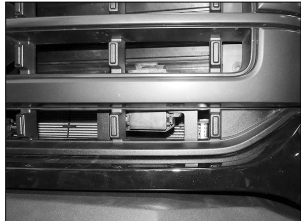
(Fig 16) Reinstall grille and plug in harness
