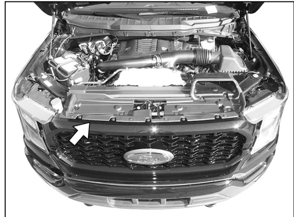
(Fig 2) Remove cover from top of grille (arrow). Remove hardware attaching top and bottom of grille and remove grille
