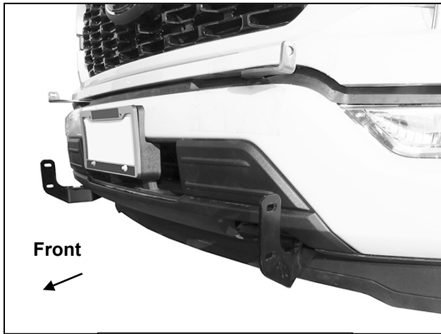
(Fig 13) Brackets installed
