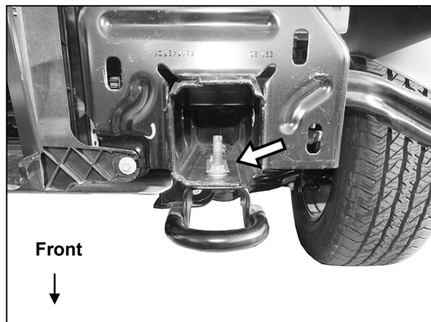
(Fig 8) Temporarily remove tow hooks if equipped
