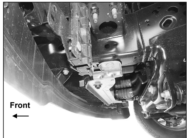
(Fig 2) Active air dam removed
