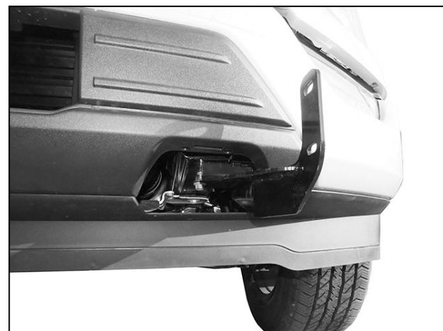
(Fig 12) Driver/left side Frame Bracket installed without tow hook
