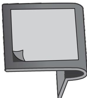
2. Place a small section of the transparent protective tape, included with the complete set, onto the flat surface of the metal bracket as shown in the picture.
