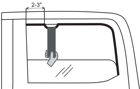
5. Bend the edge of the rubber seal from the front frame of the window by 2-3 inches. Place the fastening bracket in the channel and return the rubber seal to its original position.
