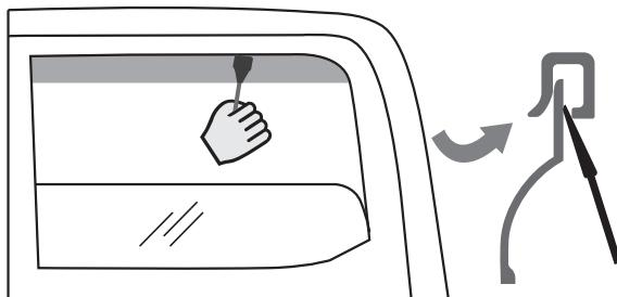
9. To ensure better installation of the deflector and better adhesion between the tape and the surface of the rubber seal, it is strongly recommended that you use the plastic blade, moving it slowly between the window's inner rubber seal and the deflector.
