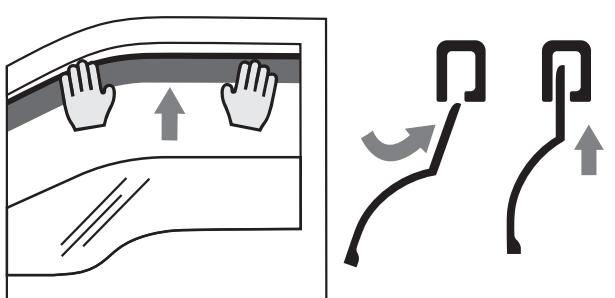
8. Starting with the front part of the deflector, insert it into the window channel.
