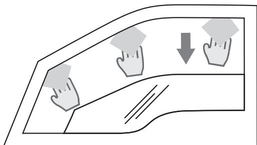
1. Make sure the car windows are clean and dry. Next, lower the side windows completely and clean the grease off the inner surface of the window channel with an alcohol wipe.
