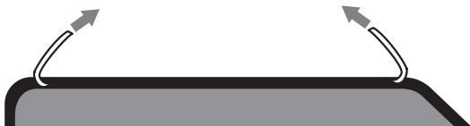
6. Remove the protective liner from the tape on the deflector.
