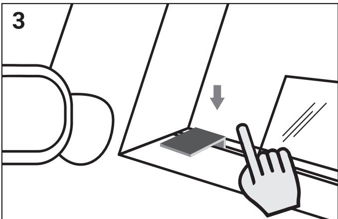
3. Place the metal bracket onto the lower rubber seal as close to the front window frame as possible.
