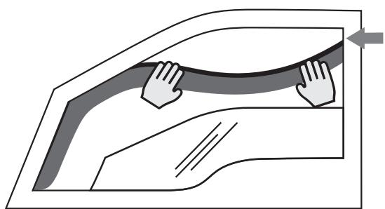
7. Bending the center part of the deflector outwards, insert the back part of the deflector into the channel, leaving a gap above it.
