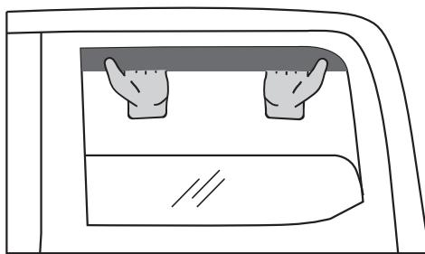
8. Immediately after installing the deflector, adjust its position by carefully pulling it outwards.
