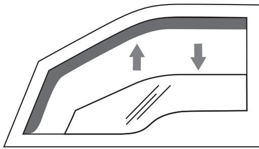
11. Raise the window until it touches the deflector. Carefully pulling the deflector outwards, roll up the window with abrupt movements. Repeat this action 4-5 times, then leave the window closed.
