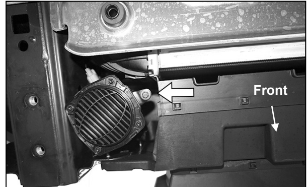
(Fig 5) Remove bolt (arrow) to temporarily remove audible alert speaker located behind driver/left side of bumper (hybrid models only-pictured from below)
