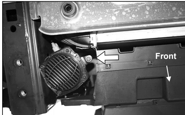
(Fig 5) Remove bolt (arrow) to temporarily remove audible alert speaker located behind driver/left side of bumper (hybrid models only-pictured from below)
