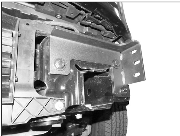
(Fig 8) Driver/left side Bracket installed
