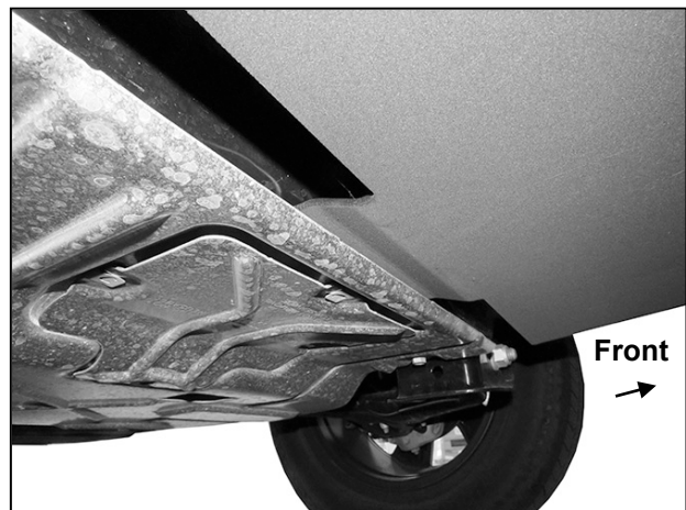
(Fig 8) Reinstall factory skid plates over LD2 Skid Plate. Large factory "off road" skid plate over LD2 Skid Plate pictured.
