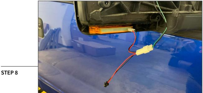
Install the supplied adapter harness. Plug the assembled plug from step 6 into the adapter harness.
