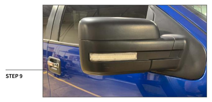
Test the light by turning on the respective turn signal. Once the light is confirmed working, follow steps 1-3 in reverse order to complete the install.
