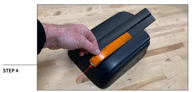
Remove the factory orange reflector from the outer mirror shell. Pry on the outer edge to unclip it from the housing.
