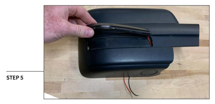
Pass the lights wiring through the mirror shell and clip the light into the mirror shell.
