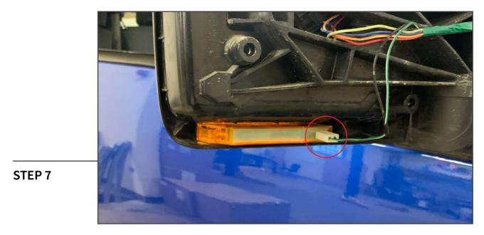
Remove the factory wiring harness from the light.
