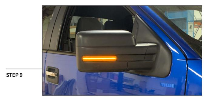
Test the light by turning on the respective turn signal. Once the light is confirmed working, follow steps 1-3 in reverse order to complete the install.
