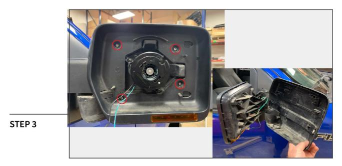
Using a T20 Torx bit, remove the (4) screws that secure the mirror shell to the vehicle. Pull the shell away from the mirror housing.
