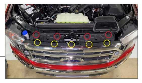
Remove (5) plastic push clips from the top of the grille. Remove (4) 10mm bolts from the radiator support to release the upper portion of the grille.
