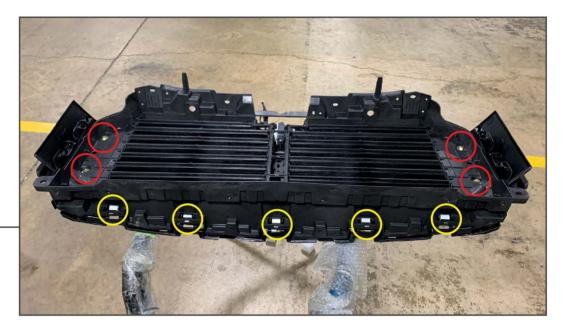
Place the shutter assembly onto the grille ensuring the (5) lower metal clips engage. Secure the shutter assembly to the grille using (4) M8x1.25 x 20mm bolts and (4) M8 flat washers. Ensure the shutter assembly is seated correctly and not overlapping the light leads.
