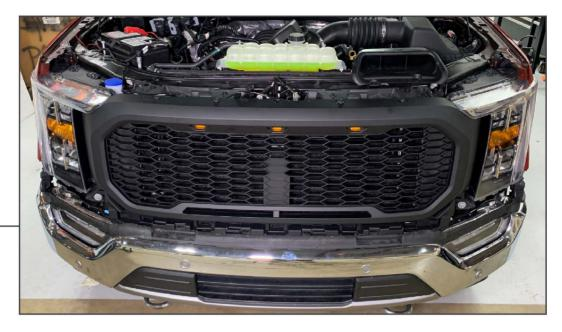
Route the LED wiring harness towards the passenger side headlight assembly. Align the grille assembly to the vehicle and secure the grille to the vehicle re-using original hardware.
