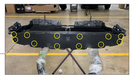
Remove (12) plastic clips from the lower portion of the grille. Remove the splash shield and set aside.
