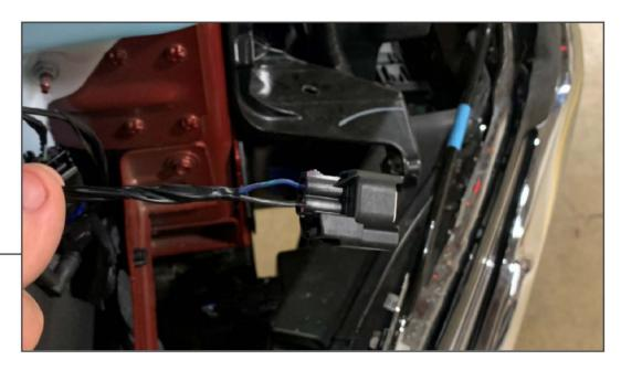
Unplug the parking light connector and tap into the circuit using (2) scotchlok conectors following the diagram below. Once the LED harness is connected, re-install the headlight following step 6 in reverse order of removal.
