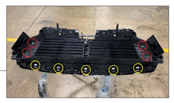
Place the shutter assembly onto the grille ensuring the (5) lower metal clips engage and the (4) M6 studs are through the shutter assembly. Secure the shutter assembly to the grille using (4) M6 flat washers and (4) M6 lock nuts. Ensure the shutter assembly is seated correctly and not overlapping the light leads before tightening hardware.
