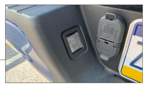
Plug the new license plate lamp assembly into the vehicle wiring harness. Ensure electrical connector audibly clicks into place. Push the new license plate lamp into the bumper light cutout.
