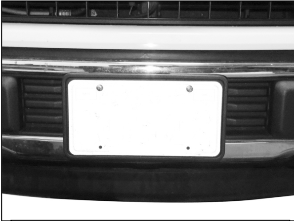
(Fig 1) Remove license plate from Bumper
