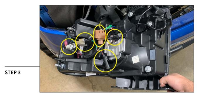
Plug in the electrical connectors into the new headlight assembly.
