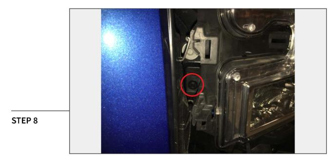
Remove (1) 10mm bolt located in between the headlight and the vehicle grille.
