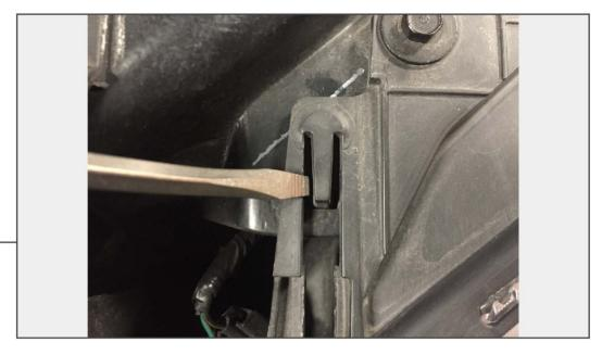
Using a flathead screwdriver, pry upwards on the locking tab while pulling the headlight forwards.
