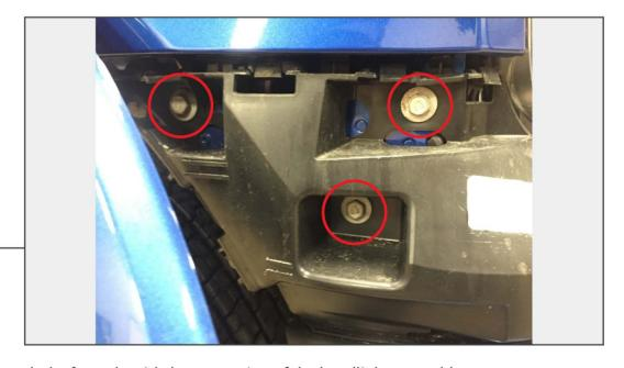
Remove (3) 10mm bolts from the side lower portion of the headlight assembly.
