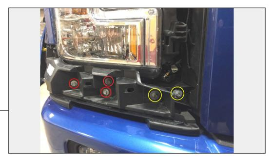
Remove (3) 10mm bolts and (2) 8mm bolts from the lower portion of the headlight assembly.
