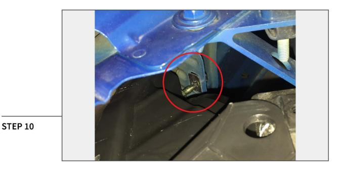
Carefully pry the headlight from the locating tab.
