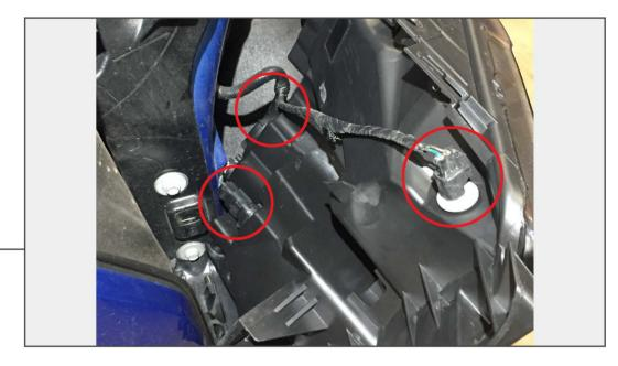
Unplug the (3) electrical connectors from the headlight, then remove the headlight from the vehicle.
