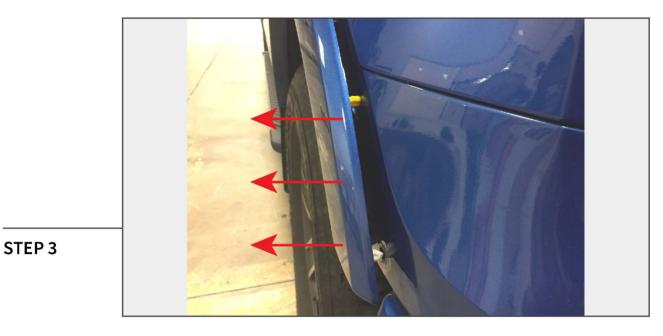
Using a panel removal tool, gently pry the fender flare away from the headlight cover.
