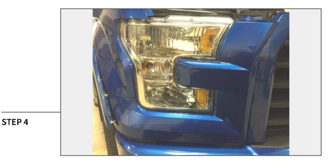
Carefully pry the headlight cover from the headlight assembly to dislodge the retaining clips. Set the cover aside.
