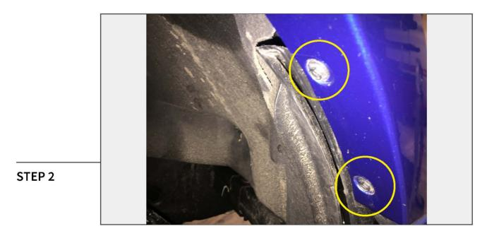
Remove (2) 7mm screws from the inner fender liner/flare.
