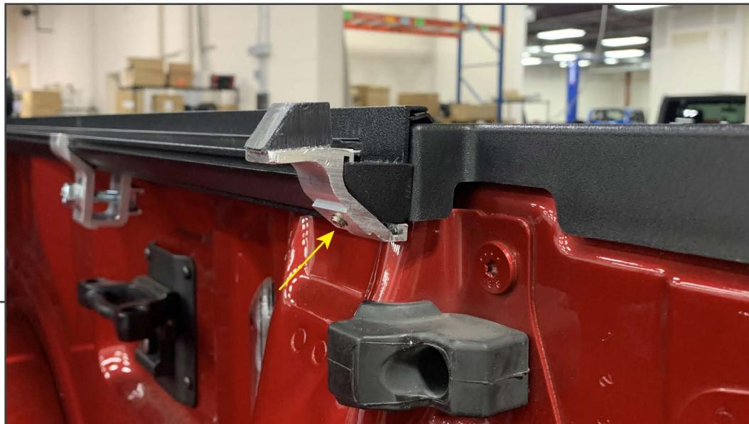
Install (1) tonneau locking bracket to the side rail. Using the Allen screw at the bottom, loosely secure into place. This bracket will be used for adjusted later.
