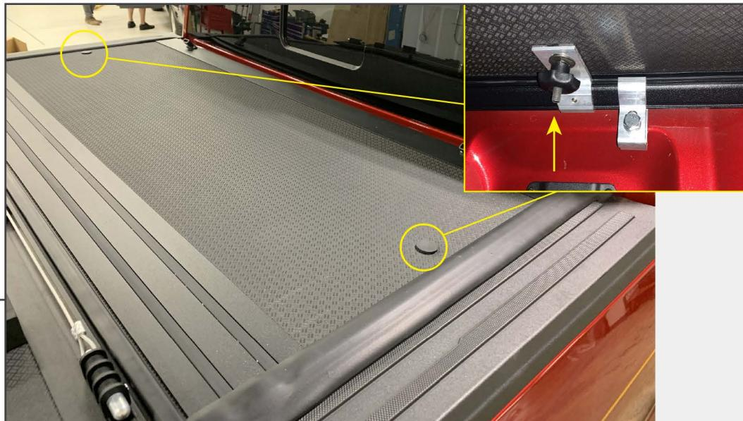
Install (2) tonneau mounting studs into the holes in the first panel on the tonneau cover, ensuring the studs go through the previously installed (2) tonneau cover mounting brackets. Secure into place using the (2) thumb screws, (2) flat washers, and (2) lock washers.
