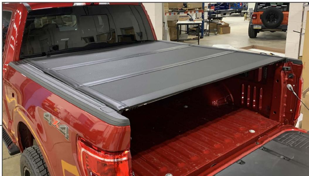
Lift the tonneau cover onto the tonneau cover side rails, ensure the cover is centered. Then, unfold the cover towards the tailgate, and adjust as necessary.
