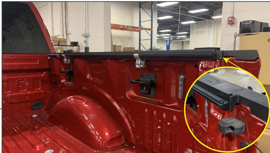
Place the side rail to the vehicle bed rail, ensuring the drain tube fitting is facing downwards and towards the vehicle cab. Align the side rail to the furthest rear point before the tailgate area. Once adjusted, tighten the (2) mounting clamps. Attach the drain tube at the front of the rail. Route the tube out of the bed using an existing hole or you will need to drill a hole to pass the tube through.
