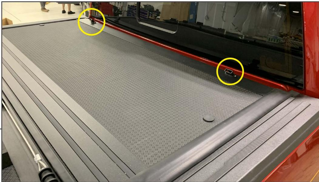
To store, fold the tonneau cover, and secure the last panel to the retaining clips using the attached straps.
