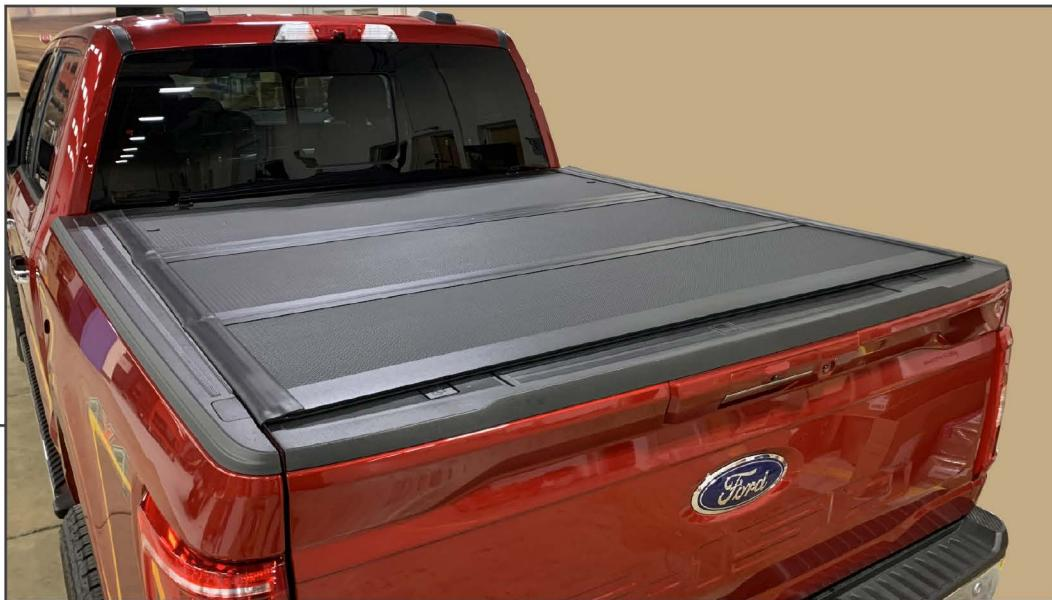
Unfold the tonneau cover and ensure the tonneau cover locks into place. Adjust as necessary to achieve desired fitment. Once properly adjusted, tighten all mounting clamps and set screws until secure.
