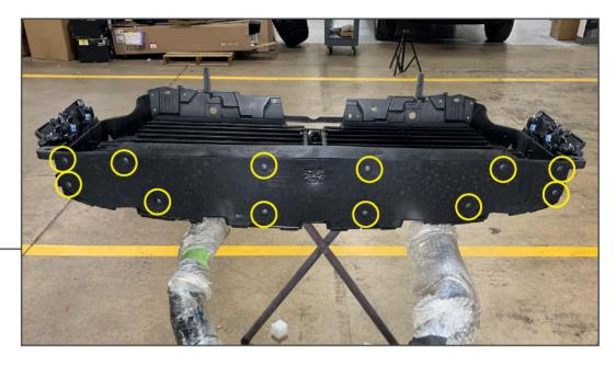
Remove (12) plastic clips from the lower portion of the grille. Remove the splash shield and set aside.
