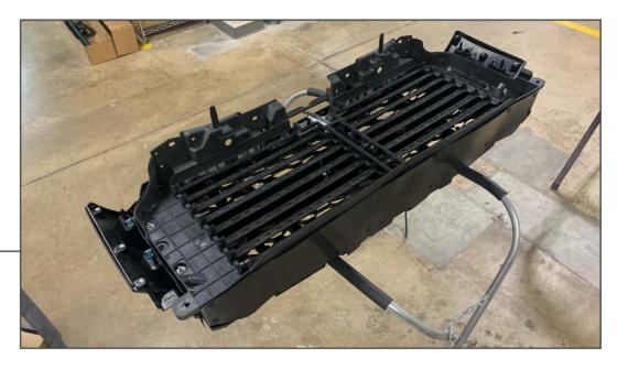
Re-install the shutter assembly and splash shield to the new grille re-using the original hardware.
