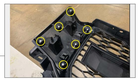
Using the appropriate included mounting panel for each side of the grille, secure the mounting panels to the grille using  $(6) \#10 \times 15 \text{mm}$  Phillips screws per panel.
