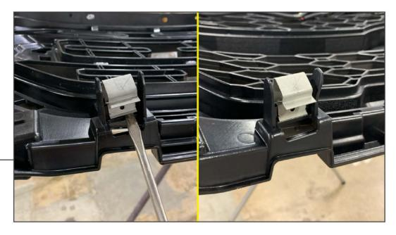
Transfer the (3) lower mounting clips from the original grille to the new grille. Removal may require gentle prying with a flathead screwdriver.
