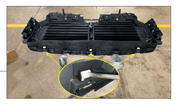
Press in the (3) metal tabs on the grille assembly while lifting upward on the shutter assembly to dislodge the shutter assembly from the grille. Remove shutter assembly from the grille.
