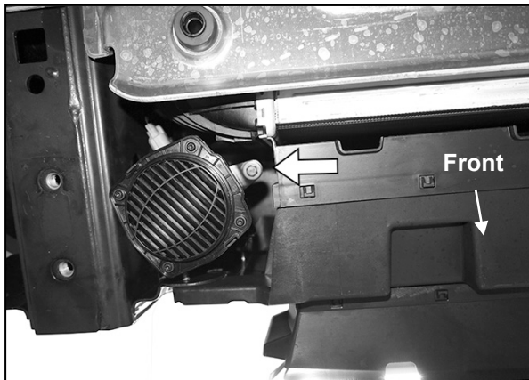
(Fig 5) Remove bolt (arrow) to temporarily remove audible alert speaker located behind driver/left side of bumper (hybrid models only-pictured from below)
