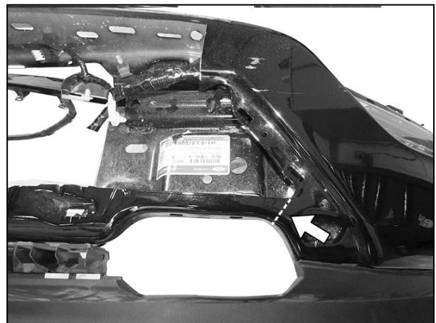
(Fig 10) Cut along dashed line (arrow). Remove air dam hardware and cut lower section
