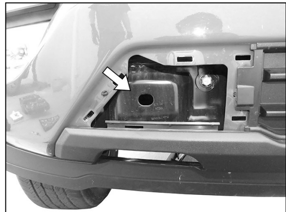
(Fig 8) Insert Bolt Plate into hole in inner bumper bracket (arrow)
