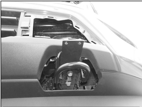
(Fig 3) Attach driver/left Support Bracket to bottom of frame, between tow hook and frame.
