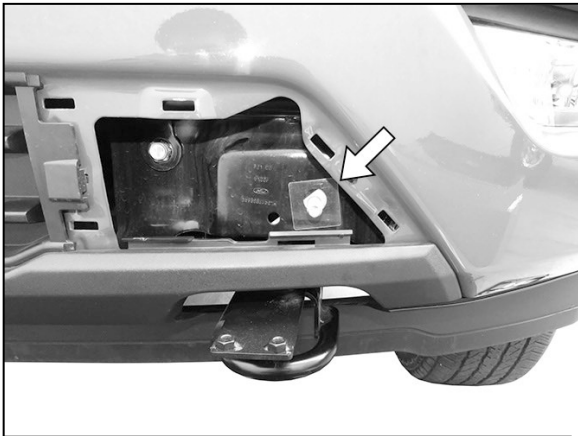
(Fig 5) Insert Bolt Plate into hole in inner bumper bracket. Thread Plastic Retainer onto Bolt Plate to hold in place (optional)
