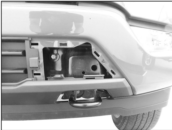
(Fig 1) Remove plastic cover from bumper. Remove tow hook and runner seal if equipped
