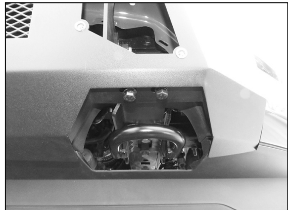
(Fig 22) Attach Support Bracket to the back of the Bumper (driver/left side)
