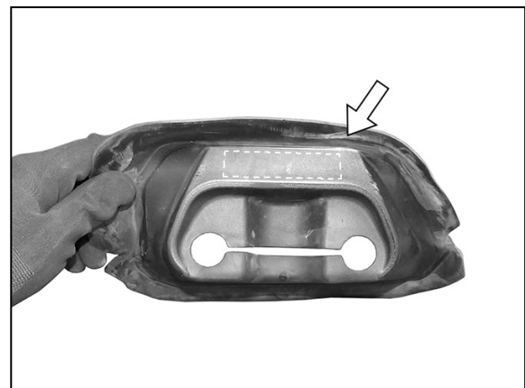
(Fig 4) Rubber seal must be cut to clear the Support Bracket, (arrow). Note, reinstallation optional
