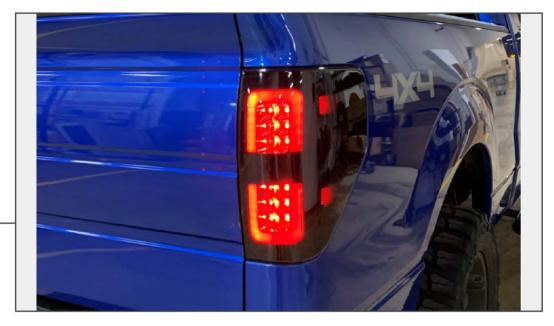
Plug in the (3) vehicle tail light electrical connectors to the new tail light. Secure the tail light to the vehicle by aligning the (2) alignment pins, then install the (2) original 8mm bolts into the side of the new tail light.
