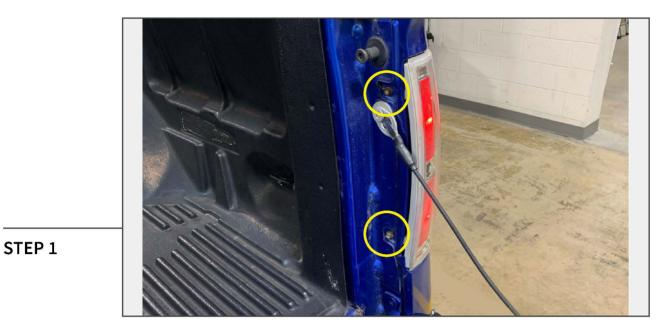
Lower the vehicle tailgate. Remove (2) 8mm bolts from the side of the tail light assembly.
