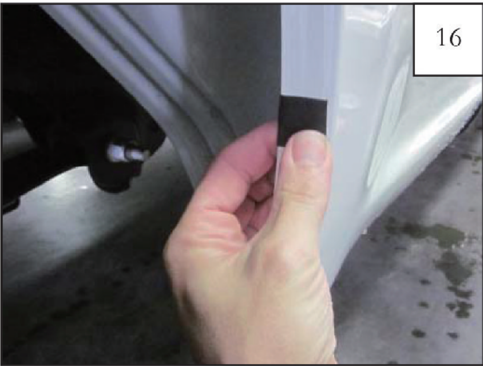
Wrap a Foam Tab (MT1-0014) around the wheel well sheet metal, centered over each of the upper four marks made in Step 15. Place a Mylar Tab (MT1-0014) at the mark made on the lower front of the wheel well.
