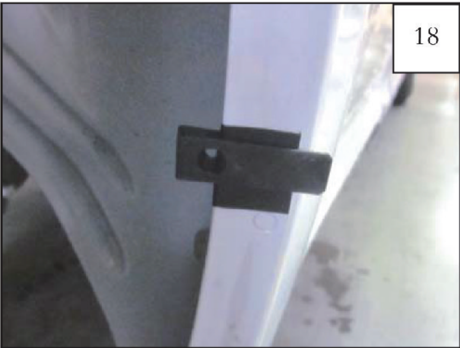
Install a Clip (CL1-0009) over each of the four Tabs (MT1-0014) placed over the upper 4 marks made in Step 16.
