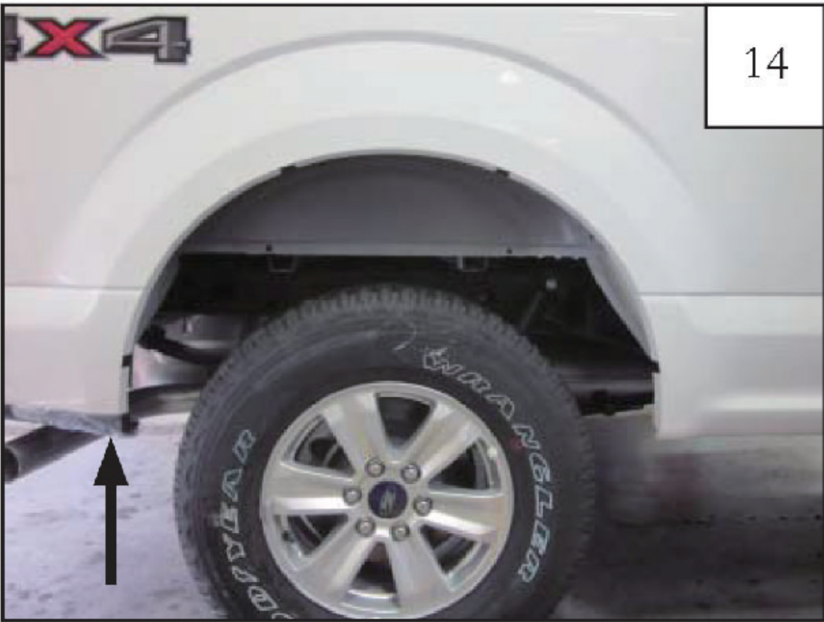
Remove factory fastener from rear of wheel well. Thoroughly clean the vehicle sheet metal and inner flange prior to installation.
