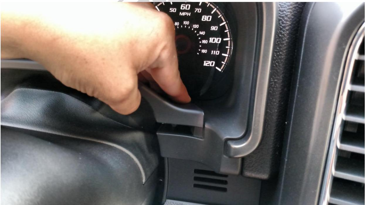
5. Next disconnect the vinyl column cover from the steering column itself. Reach under the backside of the cover and gently pull up, it will disconnect from the steering column rather easily. Completely remove this piece.
