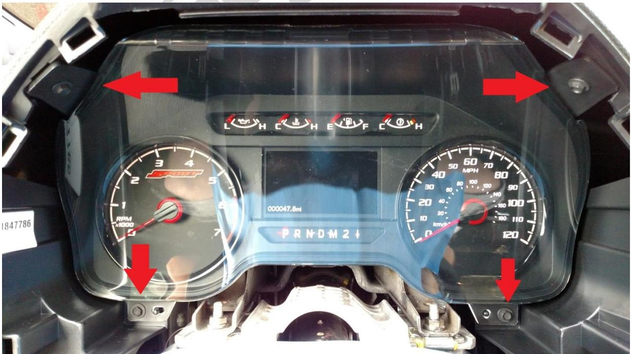
10. Slide the I/C out and remove the connector from the back side. Press the tab in the middle above the arrow and remove. Slide Instrument Cluster out.
