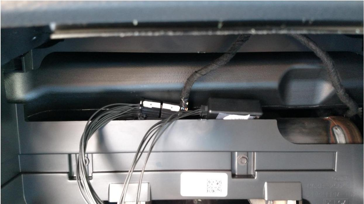
13. Slide I/C back into cavity and insert the Inline Speedometer Module harness into the I/C.
