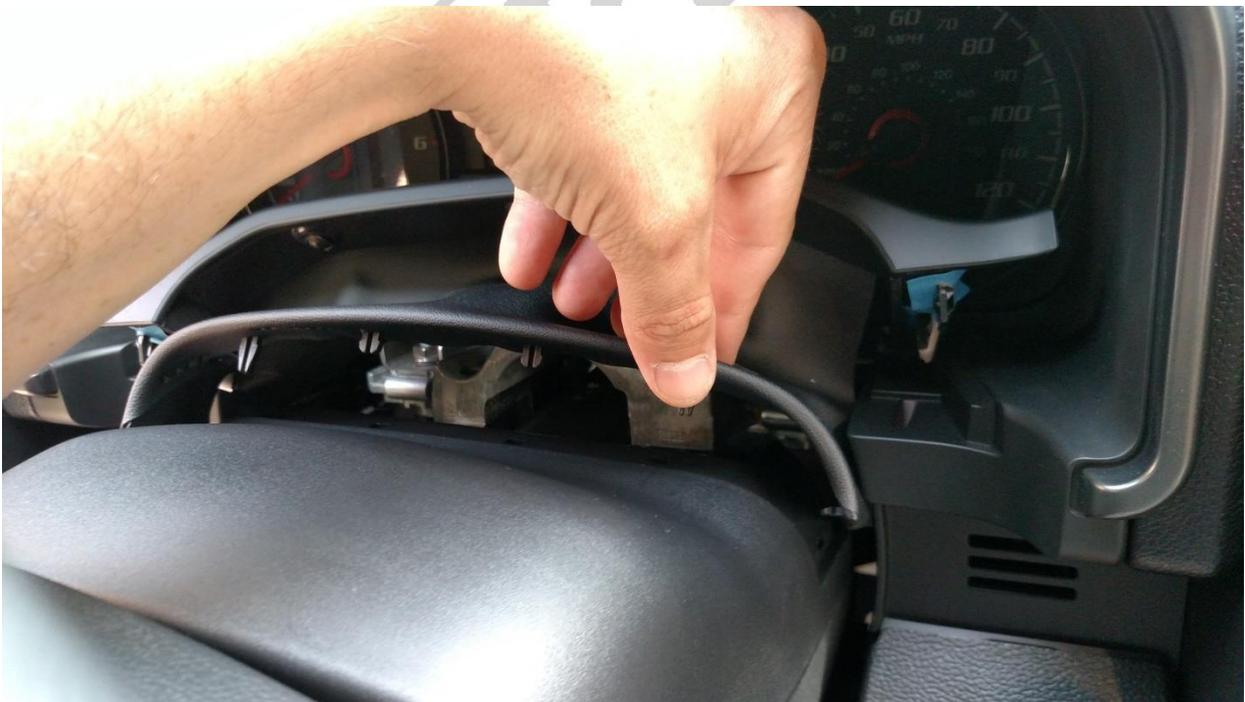
6. Raise steering column up to the highest position and reach behind the kick panel on the left and right side of the column and pull towards you to disengage the upper retaining clips. This allows access to the screws that retain the I/C Shroud.
