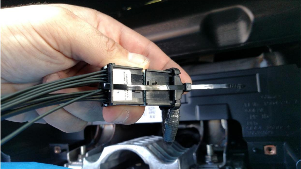
12. For the F150, tuck the harness and module on top of the air duct that runs inside of the I/C cavity to gain clearance for installation. For the F250, access to the top of the duct is limited so insert the harness and module below and orientate them sideways.
