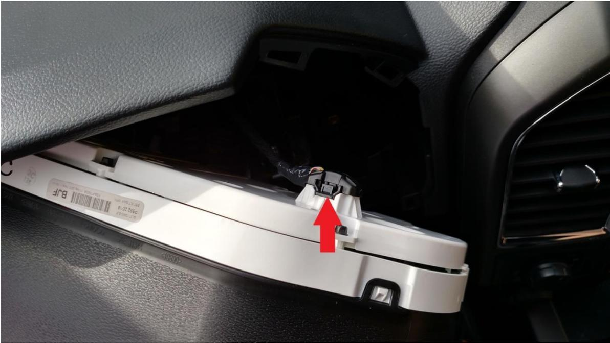
11. Plug the male side of the In-Line Speedometer Harness into the Factory I/C Connector as shown. **Make sure that the locking tabs are both facing upright and slide a zip-tie through the retaining tabs and through the hole on the bottom of the Inline Harness Connector to ensure they do not become disconnected.**
