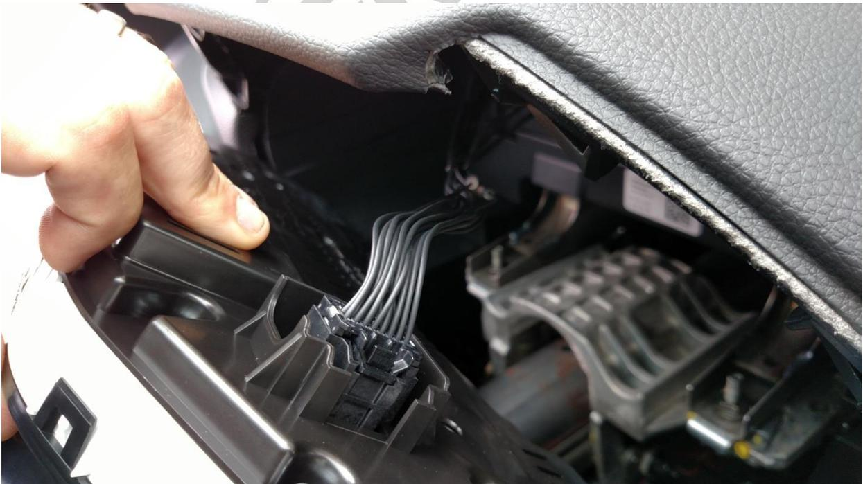
14. Install Instrument Cluster and Dash Trim in reverse of removal process. Be gentle with the vinyl steering column shroud cover, the retaining pins are easily deformed.
