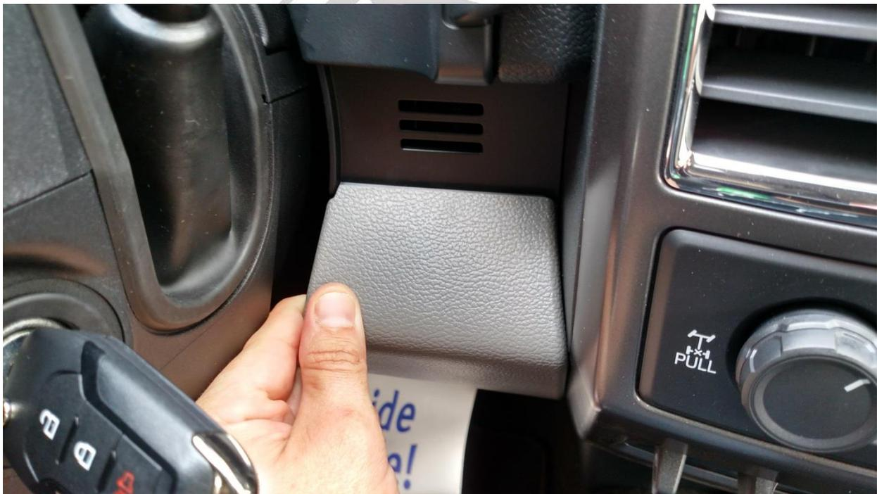
7. With the kick panel lowered, remove the (2) 7mm screws that retain the I/C Shroud.
