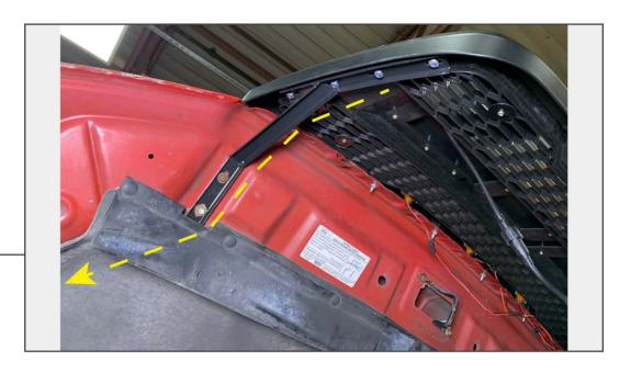
Neatly route the wiring from the grille towards the back of the hood, and then down the fender to reach the headlights. Remove each headlight and wire the grille LED lights into the vehicle following the provided diagrams.
