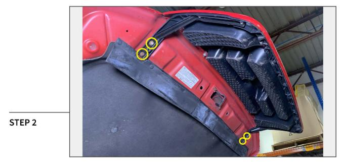
Remove (2) 10mm bolts securing the grille mounting brackets to the hood. Remove the grille from the vehicle.
