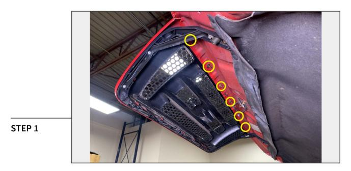
Open the vehicle hood. Remove (6) 10mm nuts securing the upper portion of the grille to the hood.
