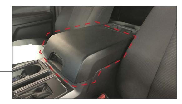
Clean the center console lid using isopropyl alcohol and a microfiber cloth. Once dry, apply the included adhesion promoter to the center console lid and allow to dry.
