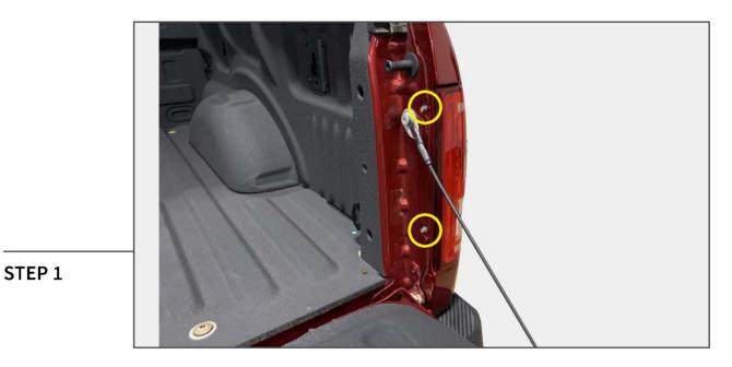
Lower the vehicle tailgate and remove (2) 8mm bolts from the tail light assembly.
