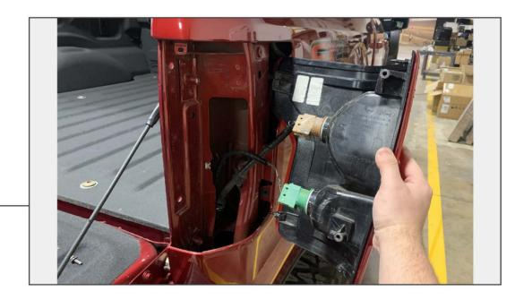
Firmly pull the tail light rearwards to dislodge the (2) alignment pins. Unplug the (2) electrial connectors from the tail light assembly.
