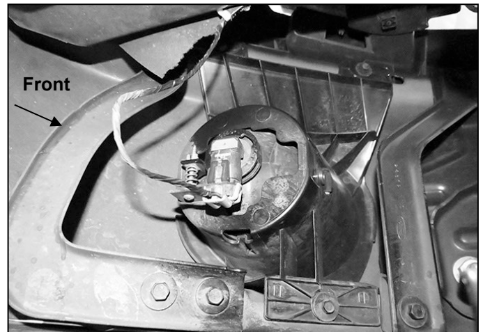
(Fig 2) Unplug factory fog light if equipped. Release clips and move wire harness away from bumper
