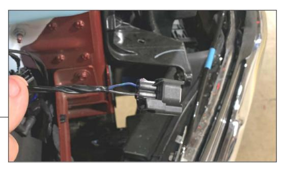
Unplug the parking light connector and tap into the circuit using (2) scotchlok conectors following the diagram below. Once the LED harness is connected, re-install the headlight following step 16 in reverse order of removal.
