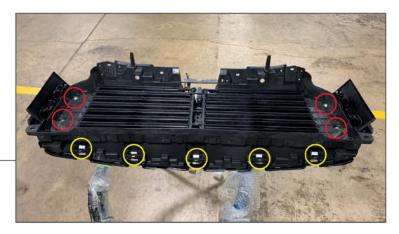
Place the shutter assembly onto the grille ensuring the (5) lower metal clips engage and the (4) shutter mounting studs are through the shutter assembly. Secure the shutter assembly to the grille reusing the original (4) 10mm nuts. Ensure the shutter assembly is seated correctly and not overlapping the wiring harness before tightening hardware. Plug in front emblem wring harness/tube, if applicable.
