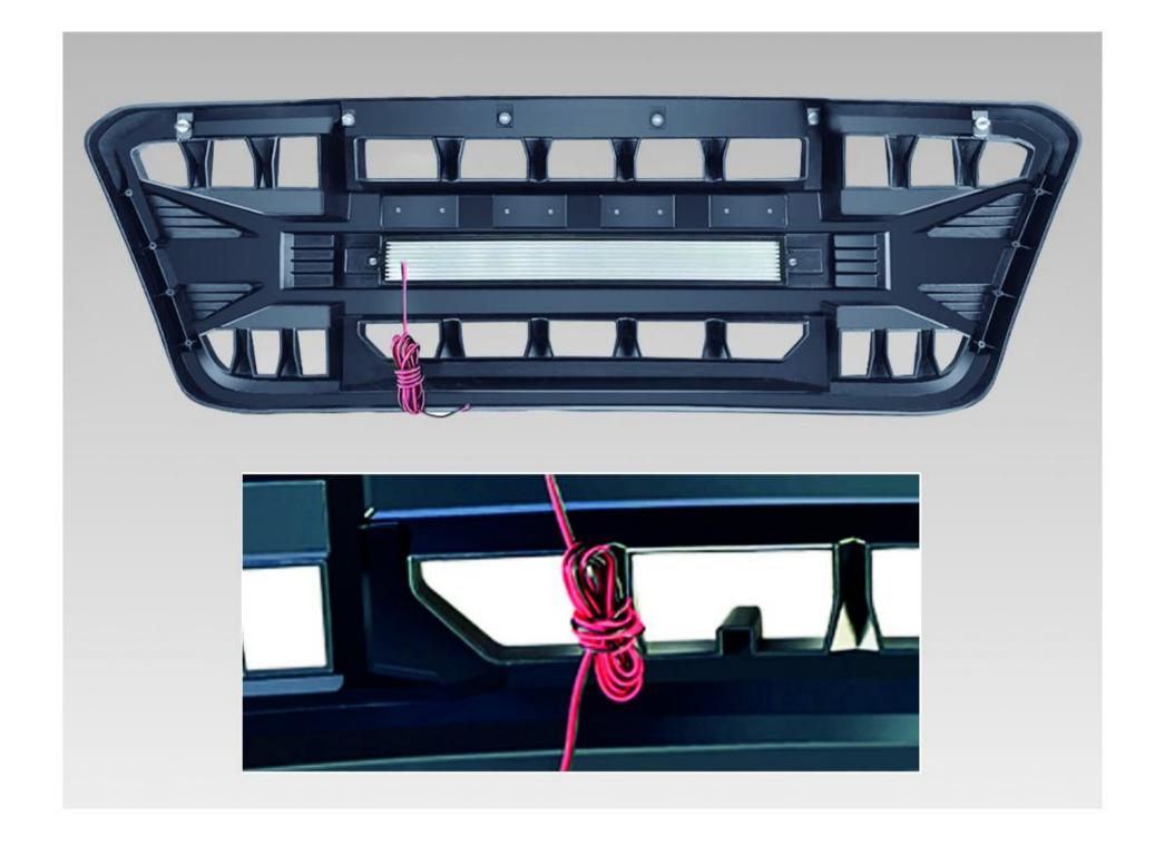
Step 3:Wiring light bar
