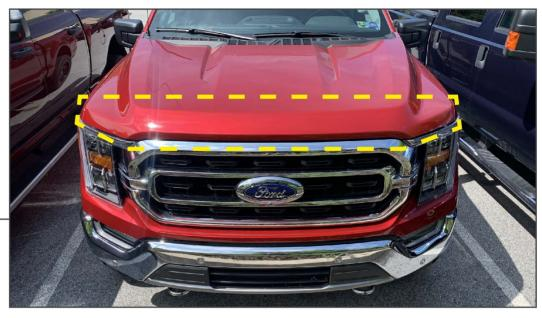
Clean the front of the vehicle hood using isopropyl alcohol and a microfiber cloth.
