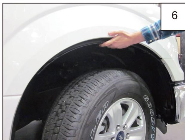
Line up the holes in the inner piece with the three uppermost factory holes. *NOTE: Both inner brackets are universal.*
