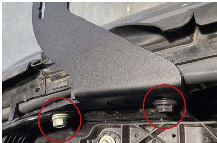
7. Remove the two 13mm bolts behind the bumper and install your new grille brackets using those mounting holes.
