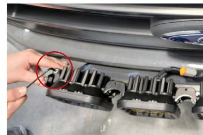
14. With all three 10mm bolts tightened down, adjust the gap on the opposite side pivot mount and secure the mount using the 5mm Allen wrench.
