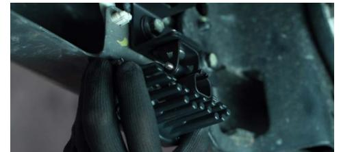
3. Install your new SSC1 or SSC2 pod onto the universal pod bracket using the provided hardware. Using a 5/32" allen-key and a 3/8" wrench, tighten the screw such that the pod retains its position, but can pivot with force for aiming.
