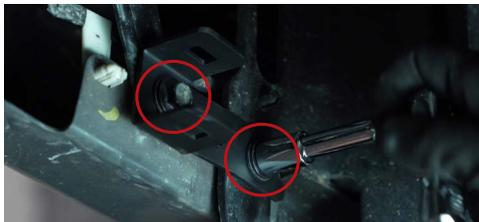
1. Using a 13mm socket and ratchet, remove the factory bolts shown in the picture above on the underside of the truck bumper. Then install your new reverse light bracket onto the vehicle using the factory bolts.
