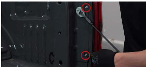
4. Drop the tailgate to gain access to the two bolts located on the side of the tail light. Using an 8mm socket, remove the two bolts holding the tail light to the truck bed.
