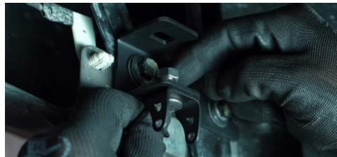
2. Install the universal pod bracket onto the reverse light bracket using the provided hardware. Make sure that the curved portion of the bracket is facing towards the rear of the vehicle.
